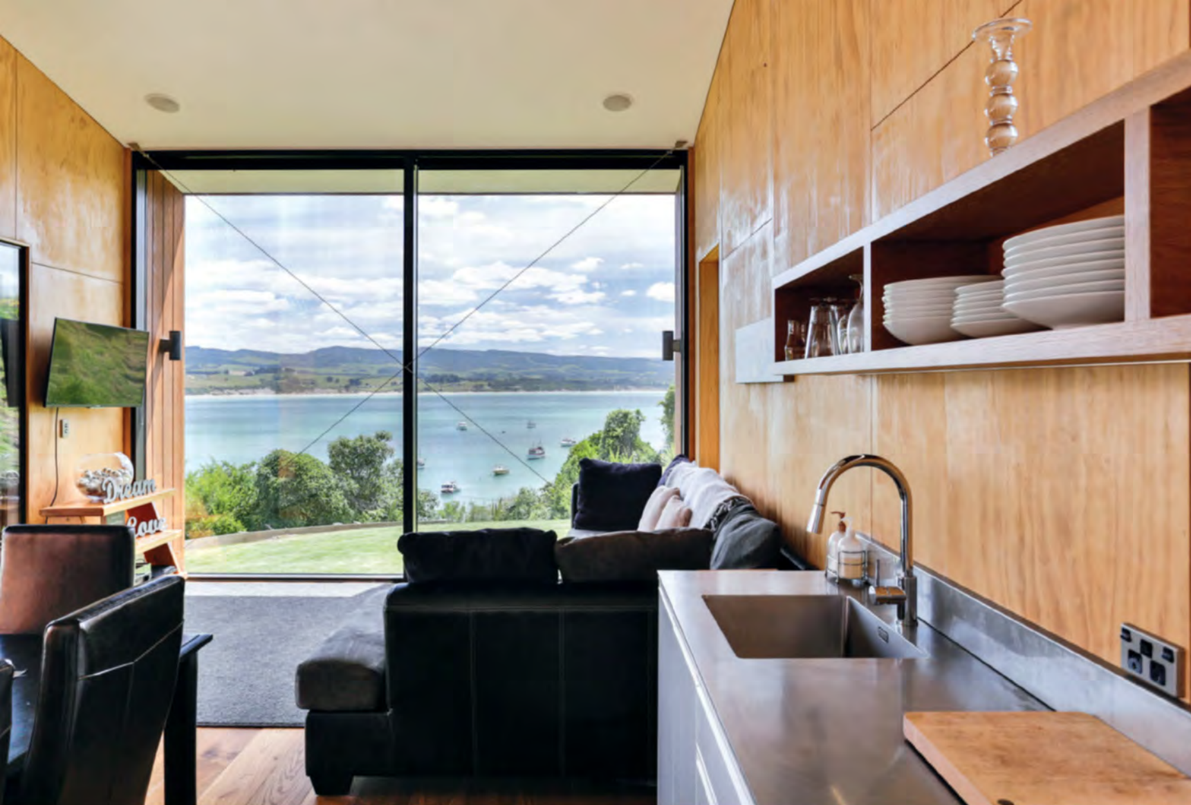
ABOVE A large picture window in the lounge had to be braced by steel cables
